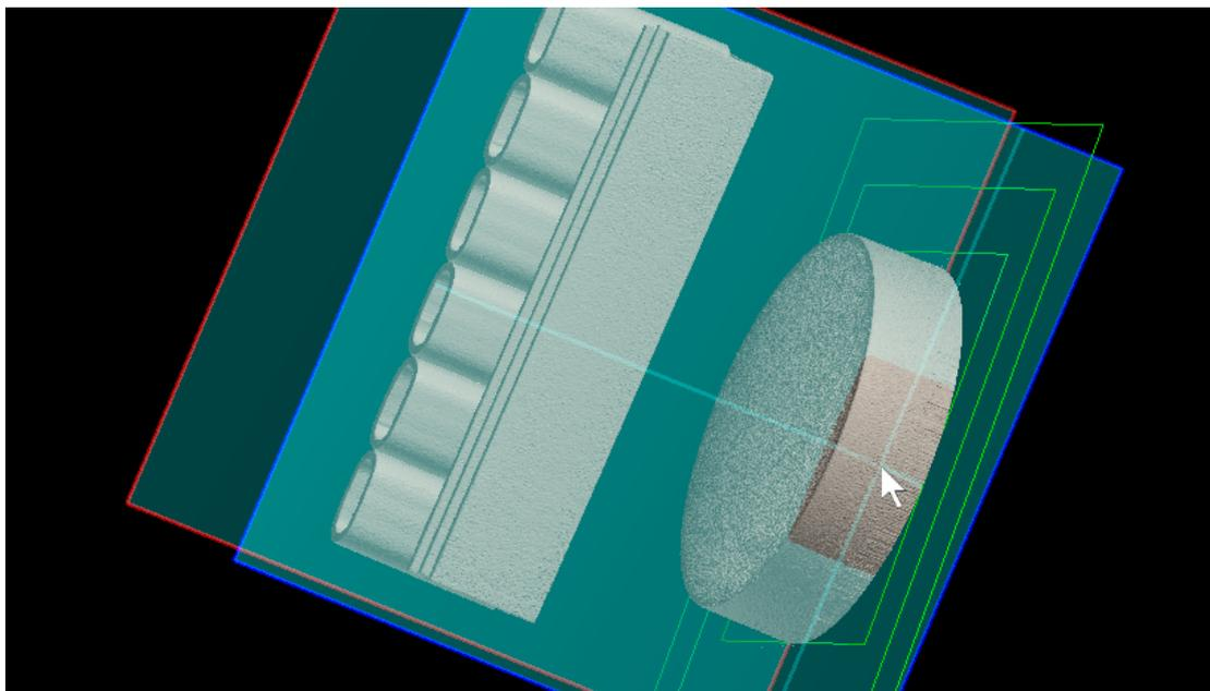
Distance between two parallel nonius planes, equal to diameter of the cylinder, is displayed in "length".
