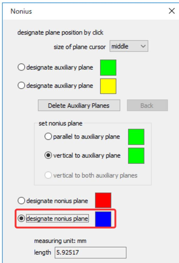
Set nonius plane (blue) in contact with curved surface like nonius plane (red).
